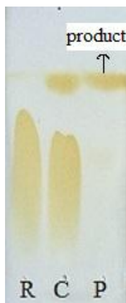
Figure 1 : Progress of the esterification reaction where R represents reactant i.e. Oleic acid, C is Co-product i.e mixture of oleic acid and the product formed and P is the Final product i.e. Methyl Oleate
