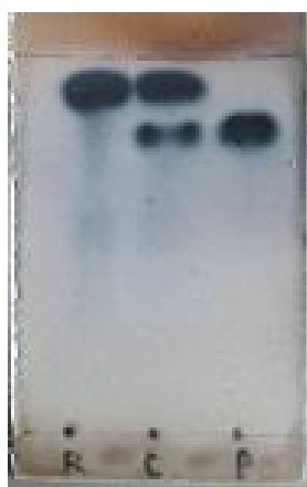
Figure 3 : Progression of the epoxidation reaction , where R represents methyl oleate, C is mixture of R and P, P is epoxy methyl oleate
