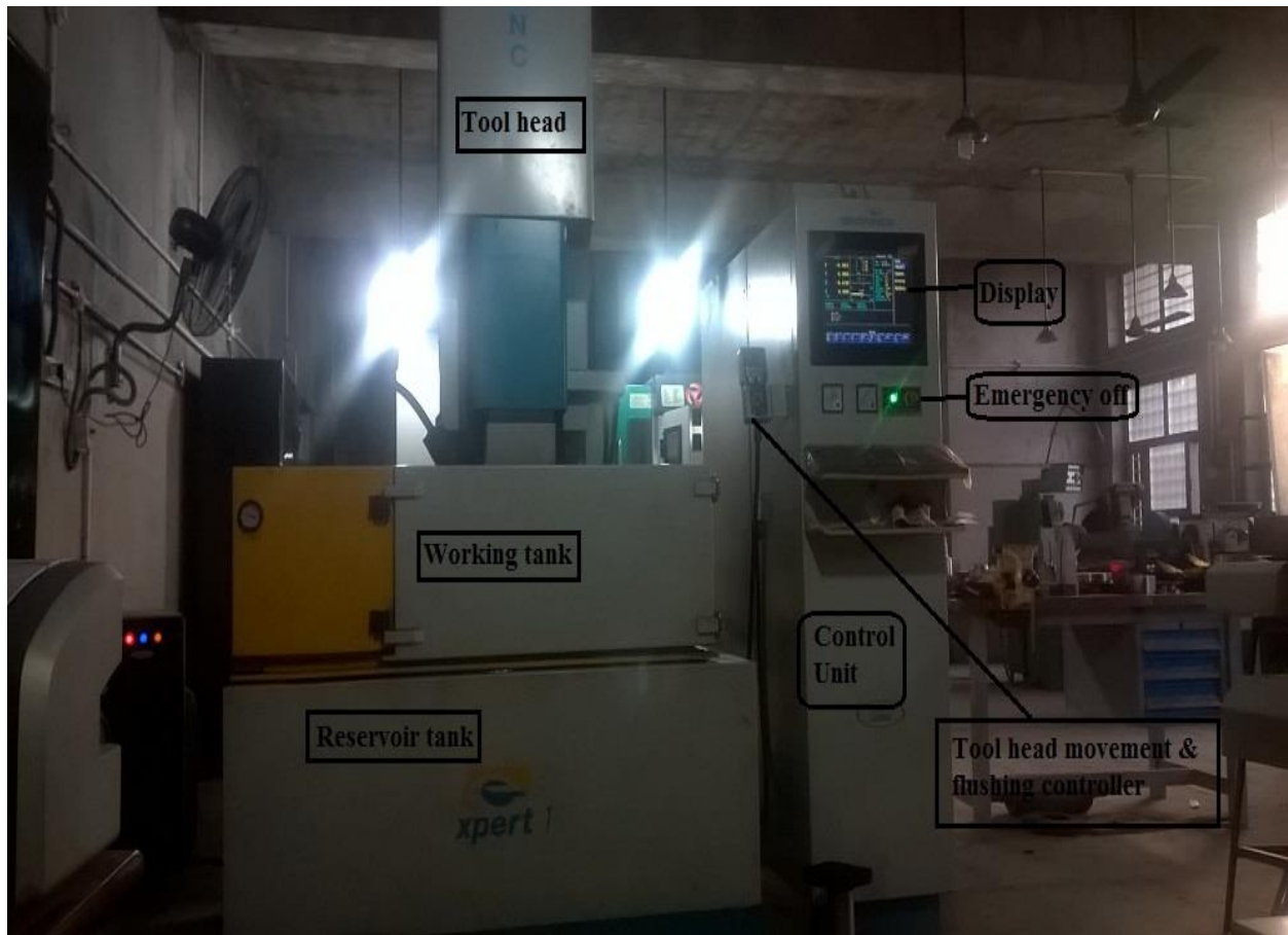
Fig 3.1 Die Sink EDM Model Electronica Xpert-1 [Global Industries, Patiala]
