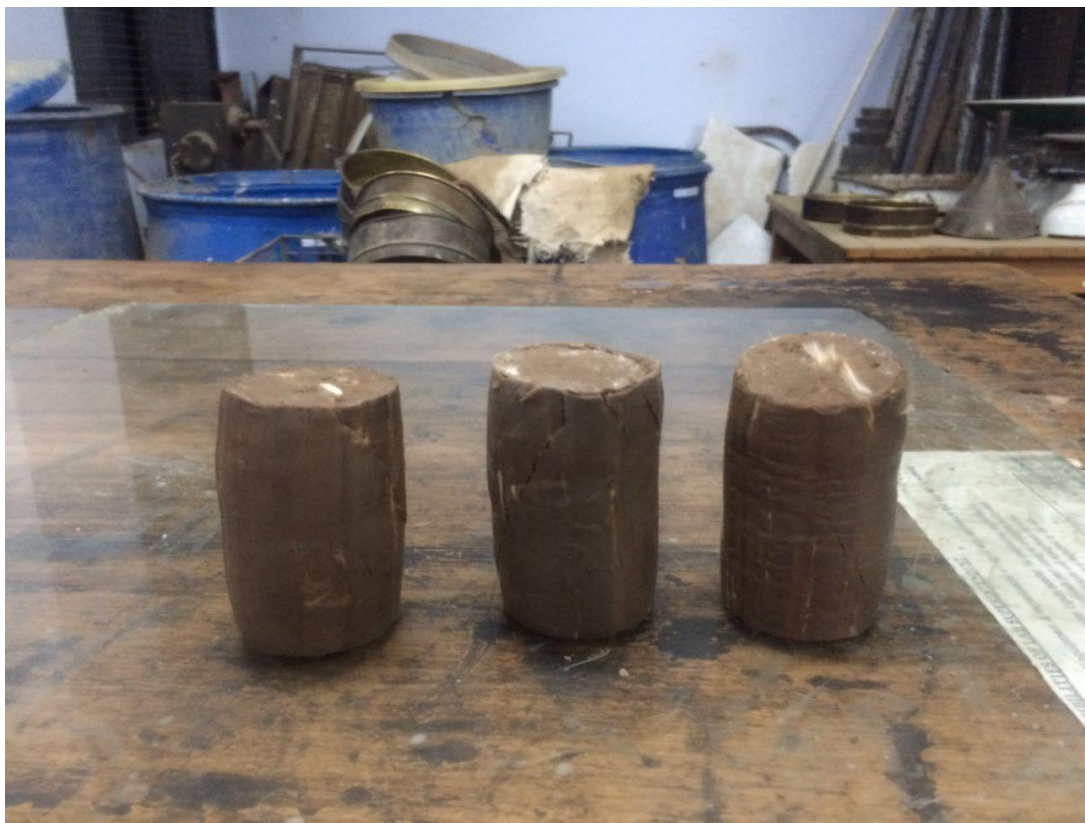
Figure 3.7: Glass fibre reinforced soil samples after triaxial test
