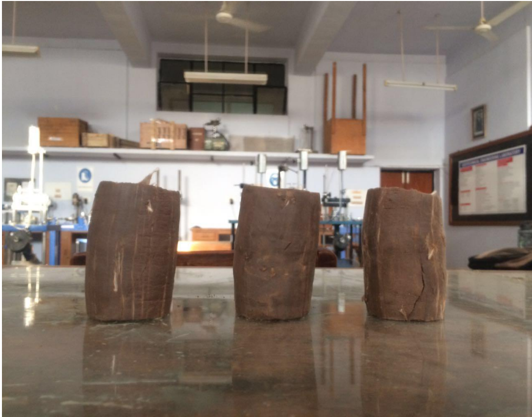
Figure 3.8: Glass fibre reinforced soil samples after triaxial test
