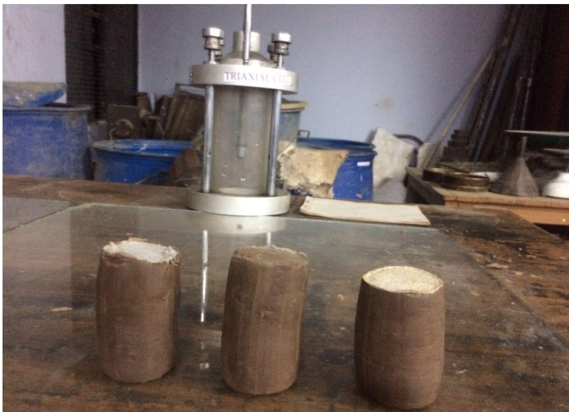
Figure 3.9: Glass fibre reinforced soil samples after triaxial test
