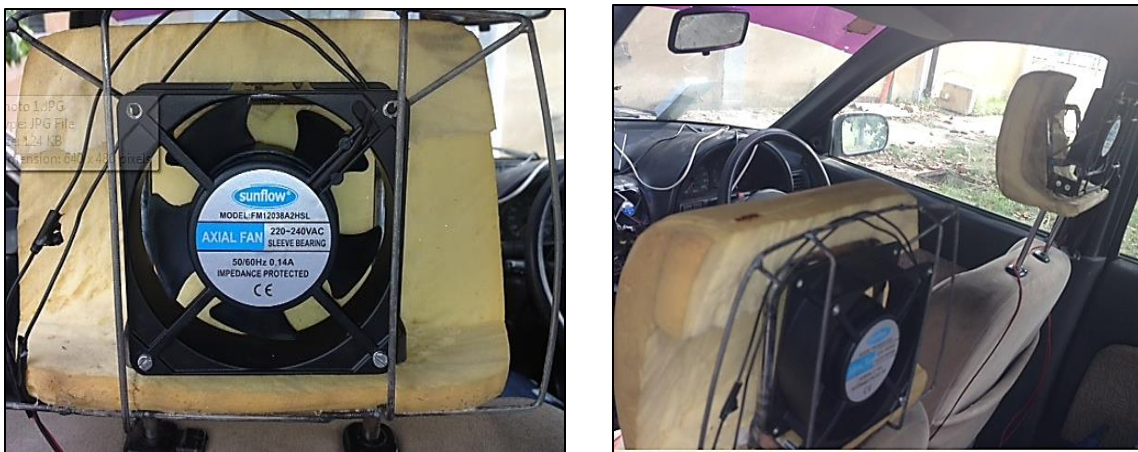
Figure 5.4: Fans installed in head rest
