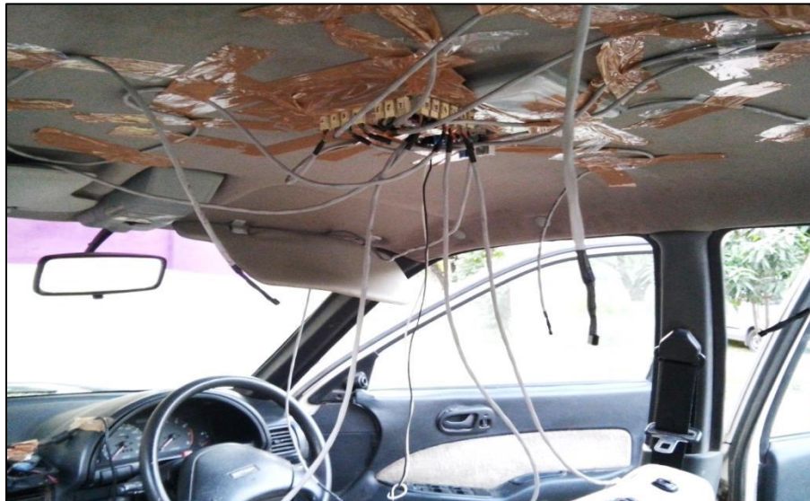
Figure 5.10: Placement of sensors and PCB
