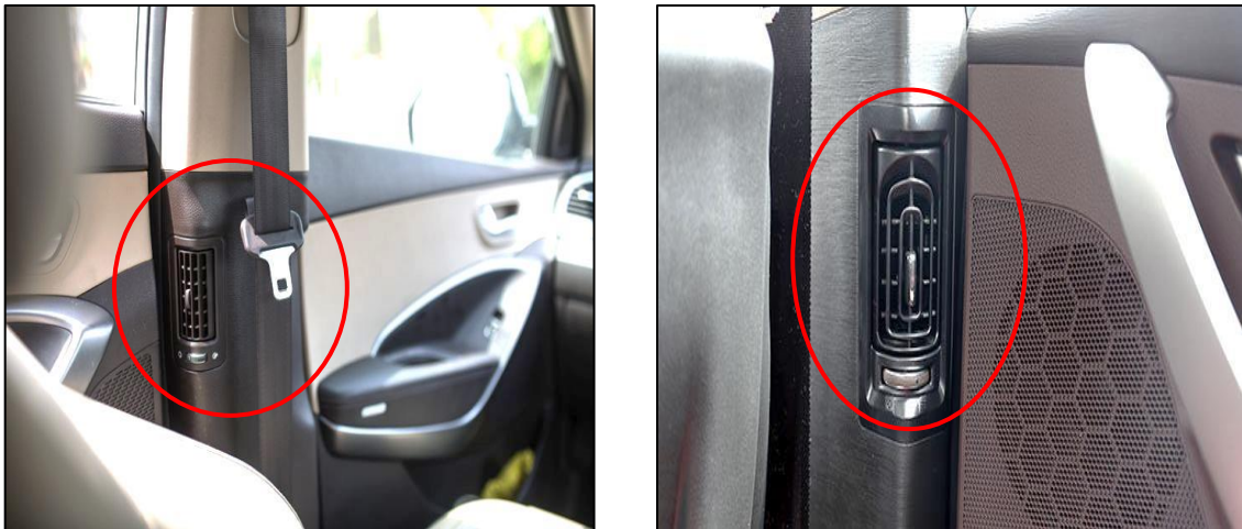
Figure 2.4: Rear vents in side pillars of car [W.1]
