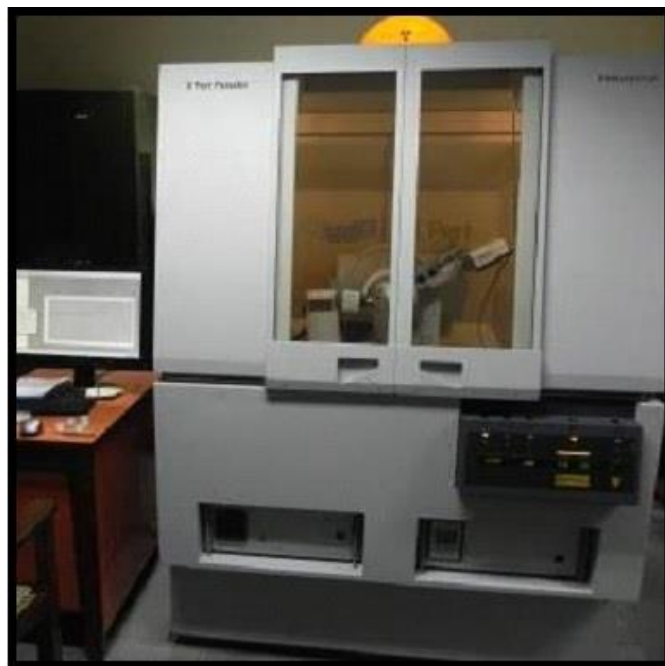
Figure 3.5: GIXRD Panalytical TM setup (Courtesy: IIT, Bombay).
