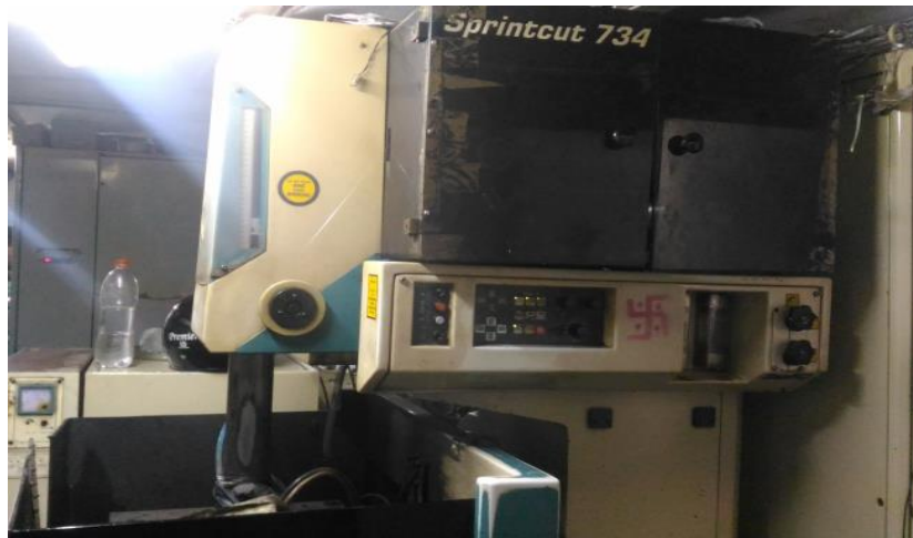
Figure 3.8: Wire EDM (Courtesy: IIT, Bombay).
