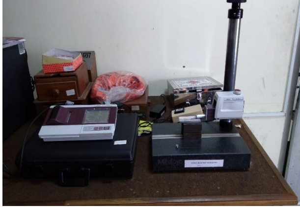
Figure 3.10: Surface Roughness Testing Machine (Courtesy: Thapar University, Patiala).
