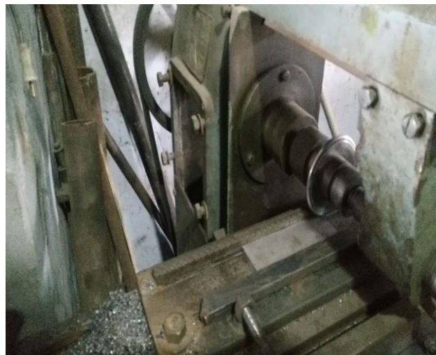
Figure 3.3: Deep rolling setup (Courtesy: Thapar University, Patiala).
