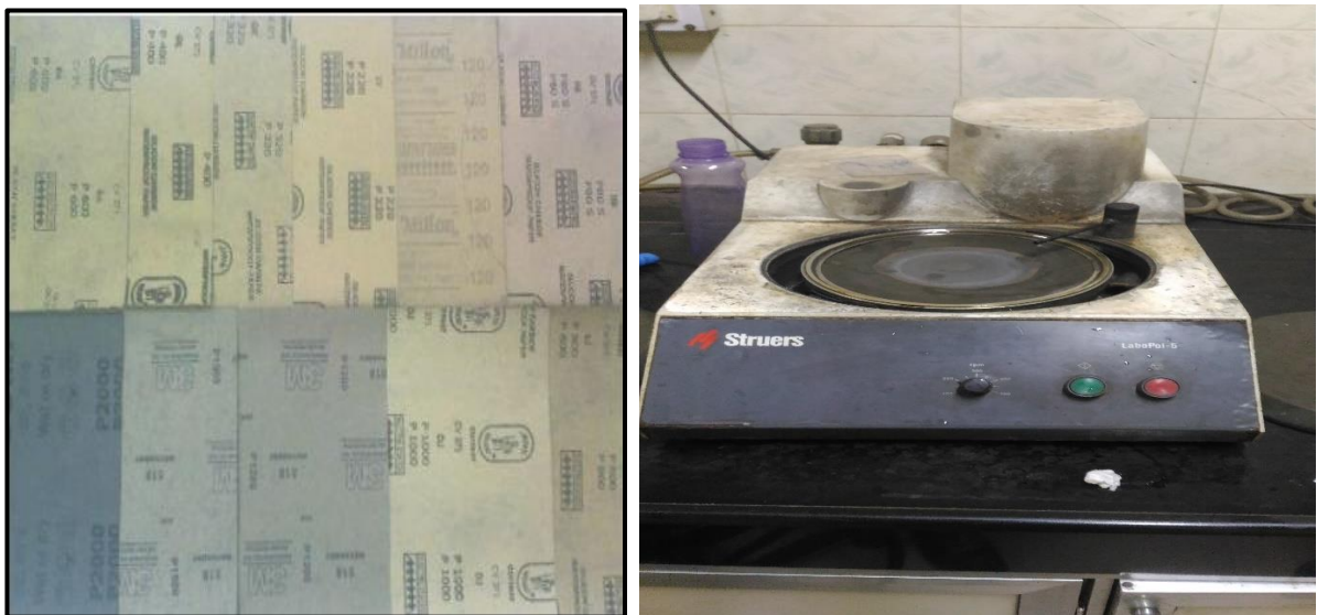
Figure 3.6: Abrasive papers and setup of grinding (polishing) (Courtesy: IIT, Bombay).
