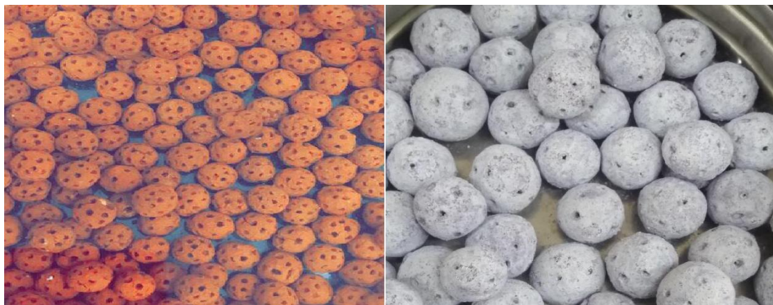
Figure 5.3: (a) Uncoated beads and (b) TiO 2 coated beads
