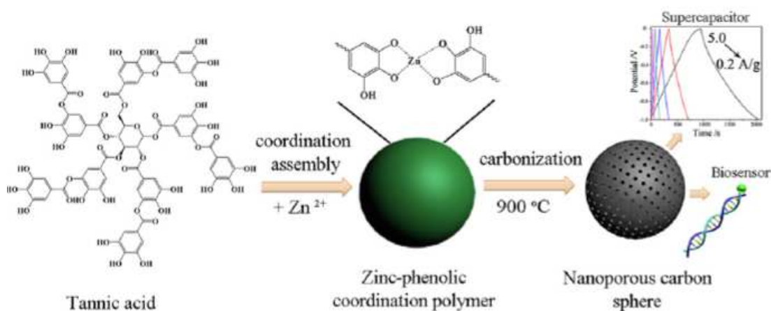
Figure 2.10: Schematic diagram CNS formation and its applications.
