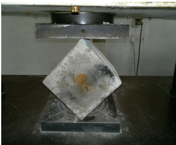
Fig.5.7 Split Tensile Test of Cube
