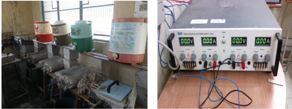
Fig 5.1 Specimens and the Power Supplies used to accelerate corrosion
