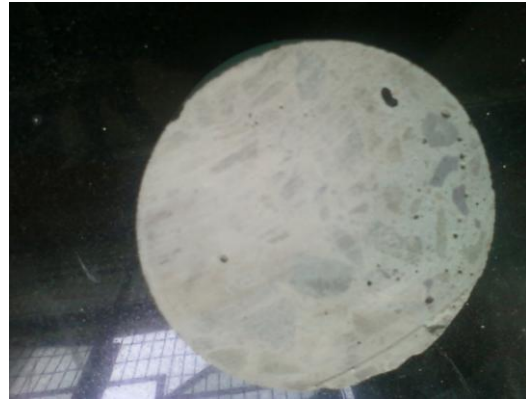
Fig. 5.9 50mm long and 100mm diameter after cutting with the machine
