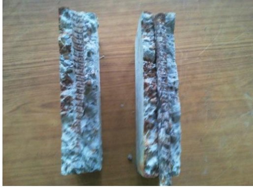
Fig.5.14 Corrosion of the rebar
