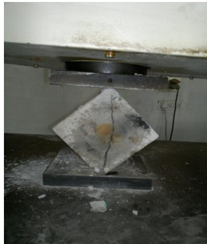
Fig.5.7 Split Tensile Test of Cube
