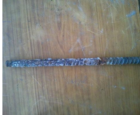
Fig.5.14 Corrosion of the rebar
