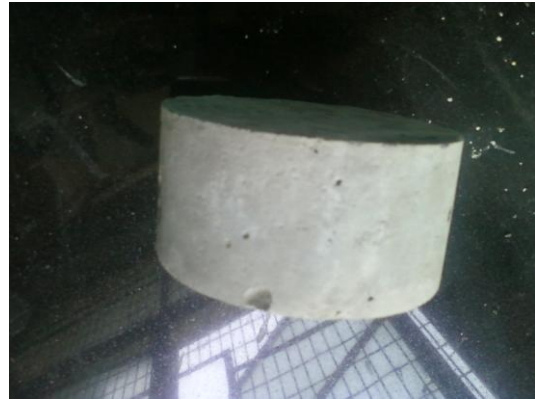
Fig. 5.9 50mm long and 100mm diameter after cutting with the machine
