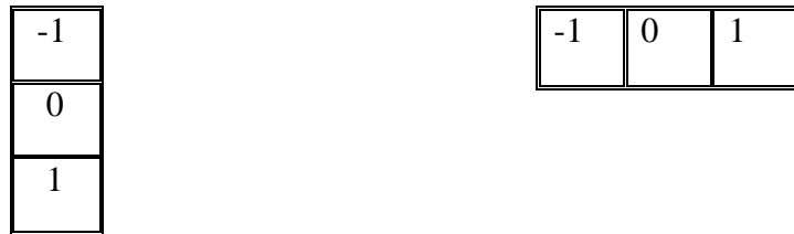
Figure 2.1: Examples of gradient kernels along: (a) vertical direction, (b) horizontal direction magnitude of the first derivative
