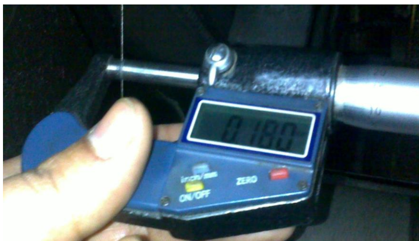
Figure 3.6 Measurement of Wire by Using Digital Micrometer
