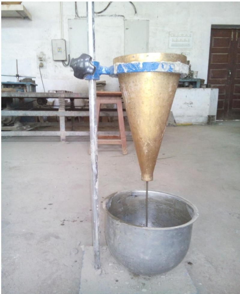
Fig. 4.4 Marsh cone test procedure
