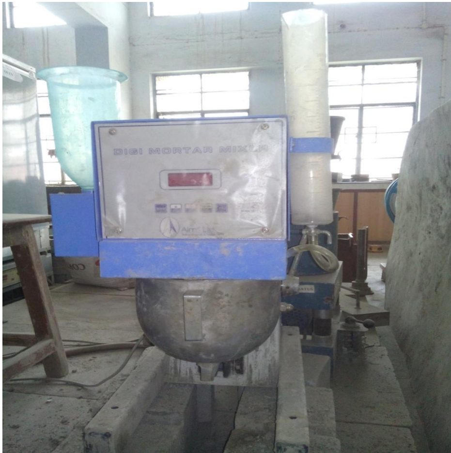
Fig. 4.5 DIGI Mortar Mixer used for preparation of cement pastes
