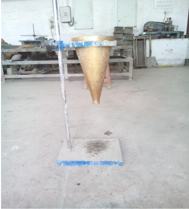
Fig. 4.3: Marsh cone apparatus used in the laboratory.
