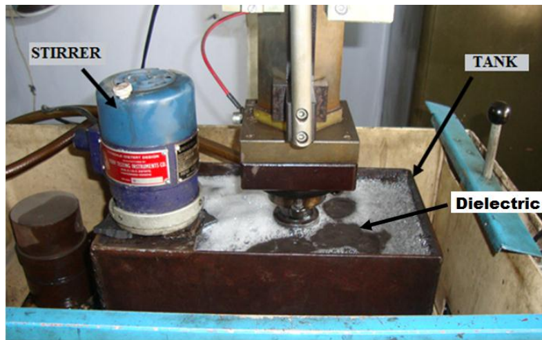
Figure 3.4: Dielectric Tank with along with stirrer
