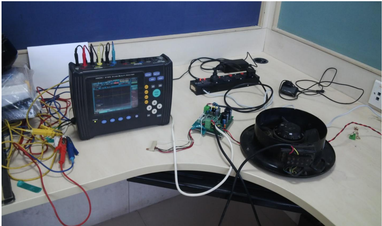
Figure 5.2: Hioki Power Factor Quality Analyzer Test Setup
