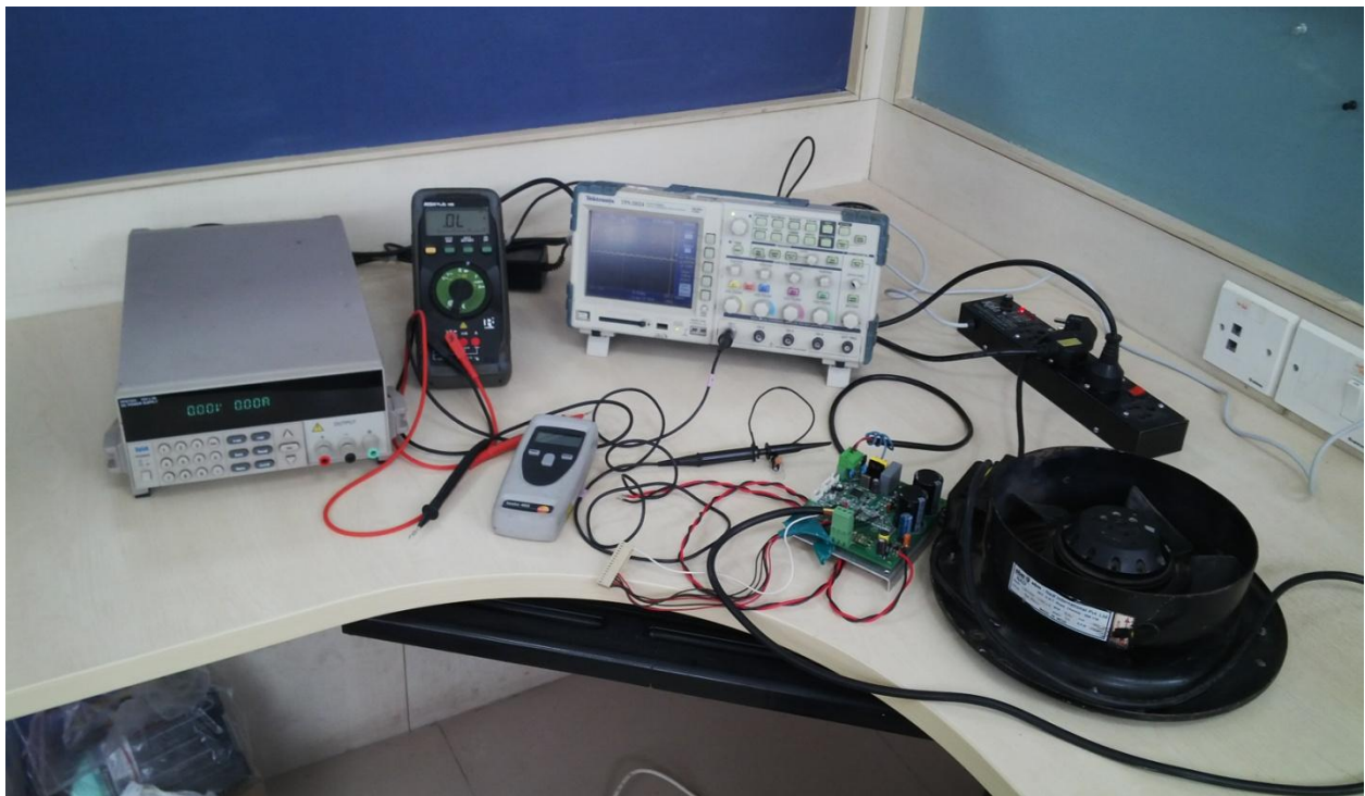
Figure 5.1: General Test Setup for Motor Control Board
