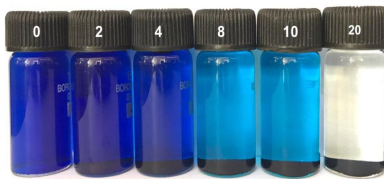
Fig 14: Methylene blue degradation at different concentrations of GO ranging from 2 mg/100 ml to 20 mg/ 100 ml
