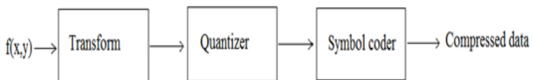
Fig. 1.6. Block diagram of encoder [1]
