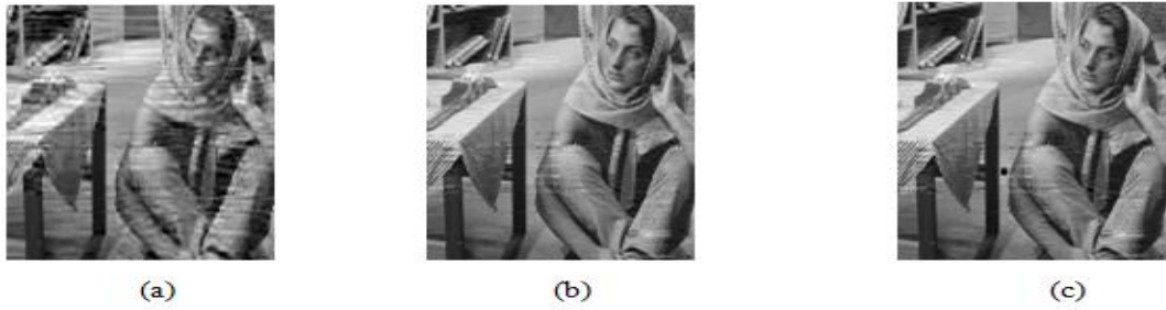
Fig. 5.62. Reconstructed Barbara images using (a) GHA (100 iterations) (b) SVD and (c) GSP
