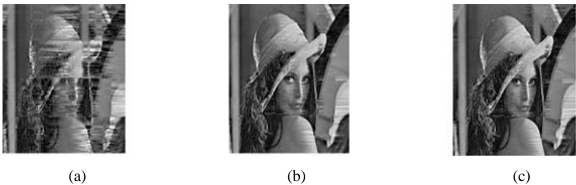
Fig. 5.58. Reconstructed Lena images using (a) GHA (100 iterations) (b) SVD and (c) GSP
